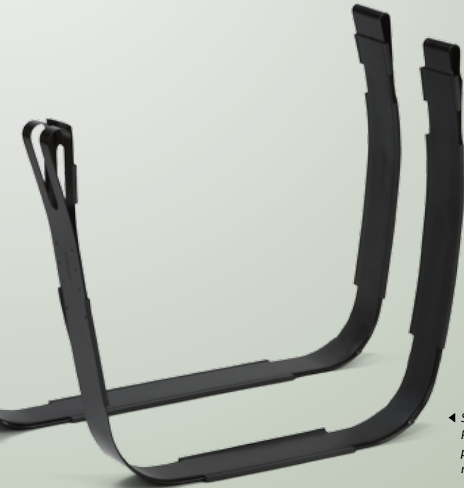
▲ Gearbox component with extremely high tolerances, produced in an 800-tonne press line with an 8-stage progression tool.
